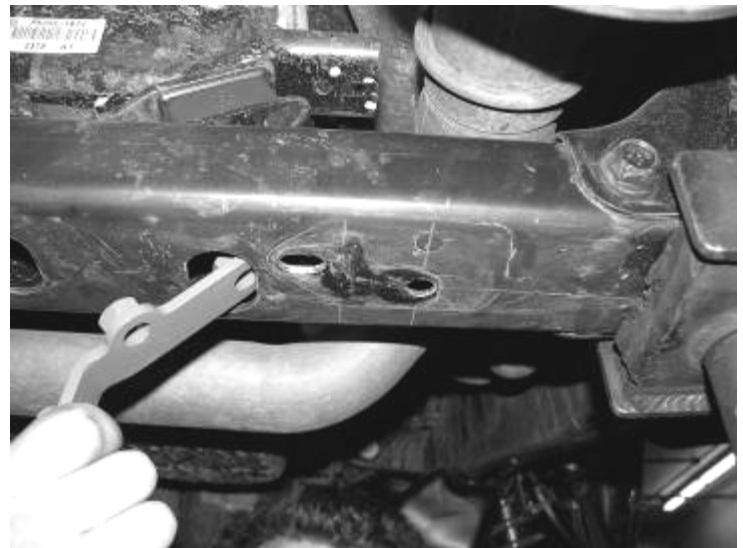
Photo Shown Installing the Nut Tab Into The Frame.
