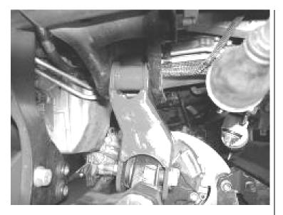
24. Place the differential housing into the Fabtech rear crossmember using the supplied ½" x 4½" bolt, nut, and washers along with the supplied large FT55-1 washers attach the differential. SEE PHOTO ON NEXT PAGE.
