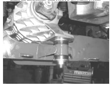
25. Locate and insert the square FT20058 tab bolts into the stock front control arm crossmember and through the holes outboard of the removed stock splash shield mounting holes. Attach the Fabtech front crossmember into the lower control arm pockets using the stock hardware. Use the 3/8" nuts and washers from hardware kit to attach the tab bolts to the under side of the crossmember. Leave loose. SEE PHOTO BELOW.
