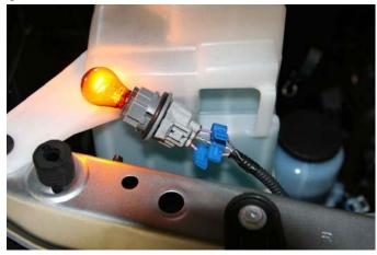
D. Tap into the OEM turn indicator harness following the color codes above.
