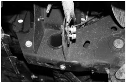
*G.* Remove the dart clips holding the rubber valance between the frame and the bumper. Also remove the two darts clips attaching the rubber valance to the grill.
