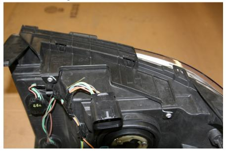
*P. With Brackets removed from the headlights skip to the next section on installation and wiring of the lights.*
