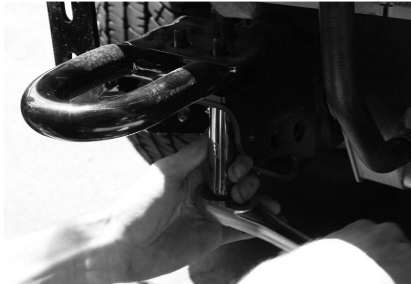
Figure 3 - Tow Hook Removal
