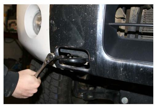
E. Using a 17mm socket remove the two bolts holding the bumper brackets to the outside of the frame on each side.
