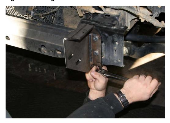
E. With mounts in Place on each side Use the help of a couple of friends to lift it into place. While in place use the supplied 7/16" Bolts, washers, lock washers, and nuts to hold in place. Do not Fully Tighten.
