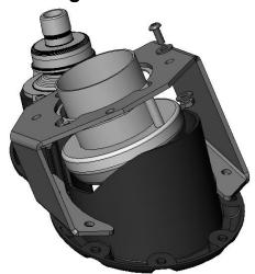
D. Install light pocket into bumper through front face, align corresponding fog lamp/bracket from back side. Secure with 10 (each side) button head screws as shown. Verify that light alignment adjusters are on bottom of light assembly. Repeat for other side.
