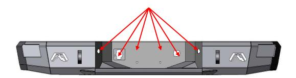
E. Install bumper mounts onto bumper as shown using supplied mounting hardware: bolts, washers, and nuts. Do not tighten fully. Verify that the triangular flange points upward and middle flange faces outward. Repeat for other side. See Image Below.
