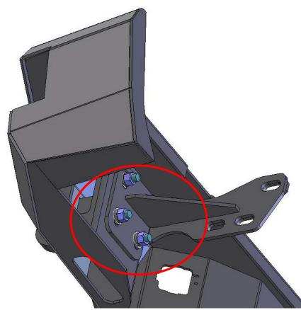
F. Align the bumper side to side and top to bottom to ensure a perfect fit to the truck. Allow for a 0.5" clearance to all painted surfaces if possible to allow for frame flex.
