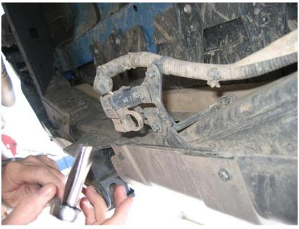
H. Remove the plastic bumper trim by prying outward and rearward simultaneously on the plastic corner protectors thereby freeing the plastic shell, set aside as it will not be reused.
