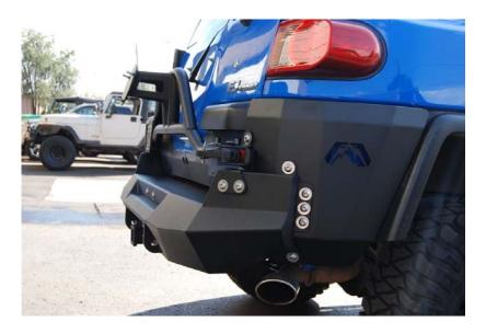
L. Once Corner Protection Pieces are aligned, retighten all fasteners loosened during Step D above.
