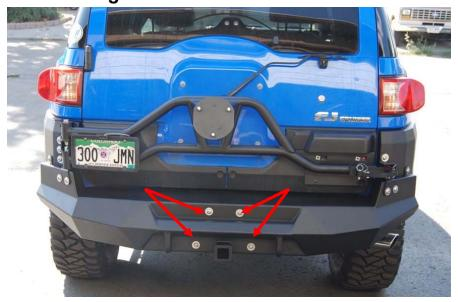
NOTE: If bumper cannot level out in relation to the truck, or is to high or low in relation to the door. Remove the bumper and re-align the Center Frame Mount (Return to Step F above).
