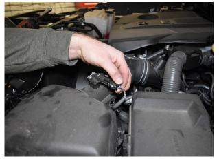
Fig. 1: Disconnect wire harness
