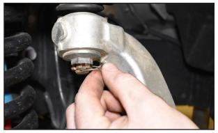
Fig. 13: Remove cotter key.
