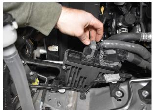
Fig. 6: PCM harness connector 2.
