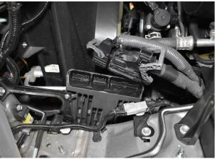
Fig. 7: PCM harness connector 3.
