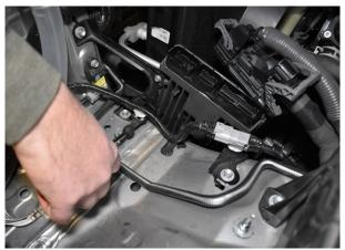
Fig. 8: Remove 3 harness clips.
