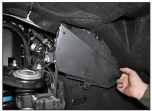
Fig. 11: Brake line shield removal
