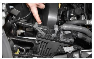
Fig. 5: Flip locking switches.
