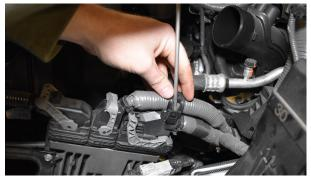
Fig. 4A: Remove PCM Clip.
