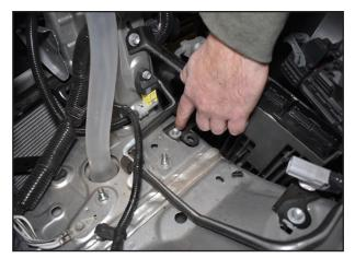
Fig. 9: Remove PCM bolts
