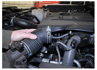
Fig. 2: Loosen the air hose clamp
