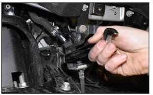
Fig. 12B: Loosen UCA hardware.
