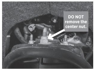
Fig. 7: Remove the three nuts, NO NOT REMOVE CENTER NUT.
