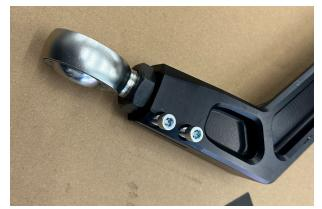
Fig. 13: Loctite and install pinch bolts.
