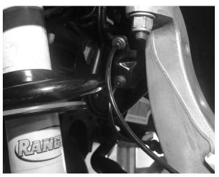
Fig. 4: Unclip ABS wire.
