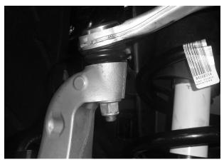
Fig. 5A: Remove nut and disconnect.
