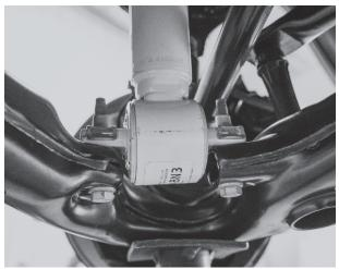
Fig. 6: Remove 2 bar pin bolts.
