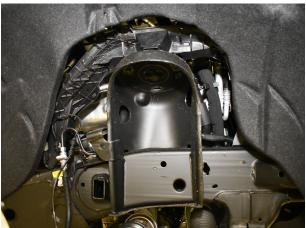
Fig. 8: Remove ABS wire then remove UCA.
