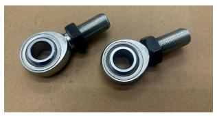
Fig. 10: Install the 3/4" jam nuts.
