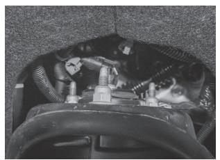
Fig. 2: Loosen the 3 upper mount nuts.
