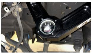
Fig. 16: Assemble uniball joint.
