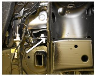
Fig. 9: Cut tab from strut bucket.
