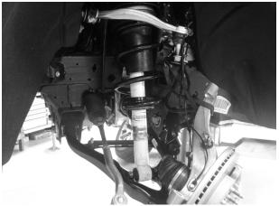
Fig. 5B: Use strap to hold knuckle.
