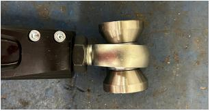
Fig. 14: Install misalignments.
