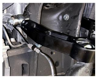
Fig. 19: Install ABS wire mount.
