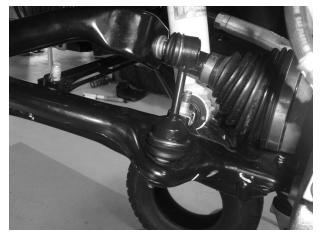
Fig. 1: Disconnect sway bar link.
