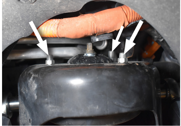
Fig.9: Remove the 3 Strut nuts.
