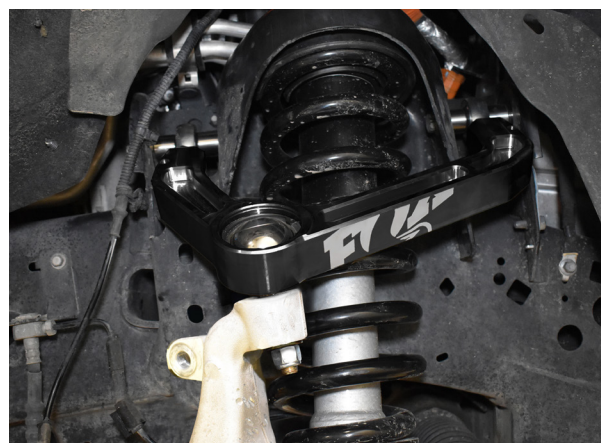
Fig. 21: Connect UCA to knuckle.
