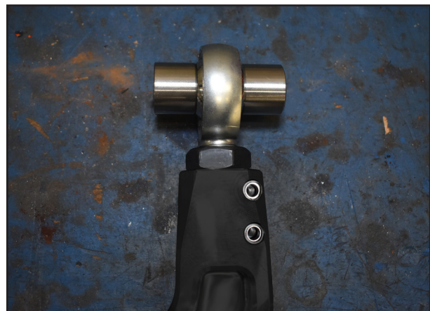
Fig. 14B: Install misalignments.
