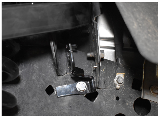
Fig. 24: Install sensor bracket to frame.
