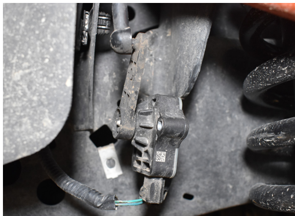
Fig. 23: Remove Sensor from bracket.
