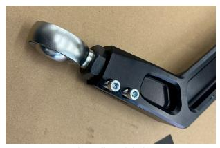
Fig. 13: Loctite and install pinch bolts.
