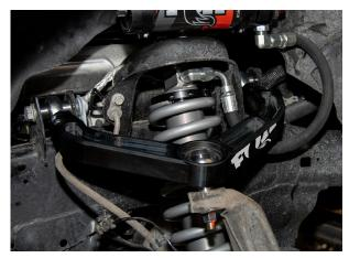
Fig. 17: Install upper control arm.
