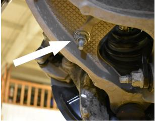
Fig.2: Disconnect sway bar link.
