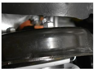
Fig. 4: Loosen the 3 upper mount nuts.
