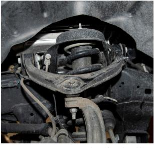
Fig. 1: Disconnect upper control arm from knuckle.
