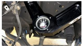
Fig. 16: Assemble uniball joint.
