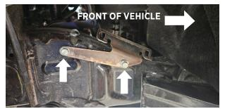
Fig. 5: Install the reservoir bracket assembly.
