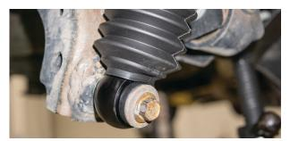
Fig. 21: Install the lower shock bolt (passenger side shown).
