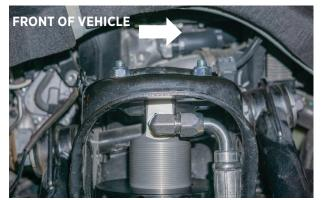
Fig. 8: The hose fitting faces outboard.
