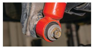
Fig. 18: Remove lower shock mount bolt.
