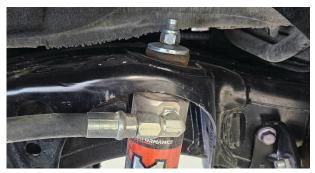
Fig. 20: Install the stem top nut (passenger side shown).
