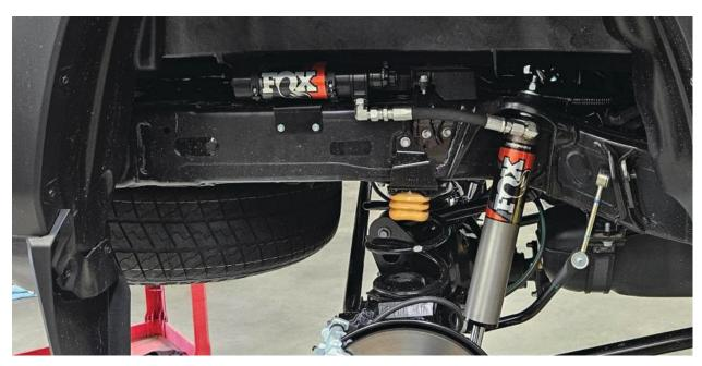
Fig. 22: Mount the reservoir to the bracket (passenger side shown).
