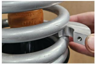
Fig. 15: Slide spacers through spring.
