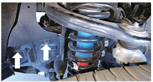
Fig. 4: Remove the plastic plugs of the splash guard.
