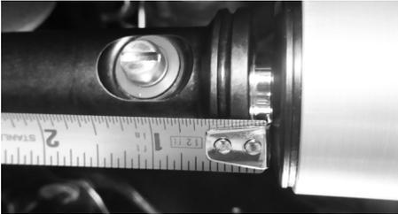
Fig. 1: Eyelet installed with 1/8" of shaft exposed
