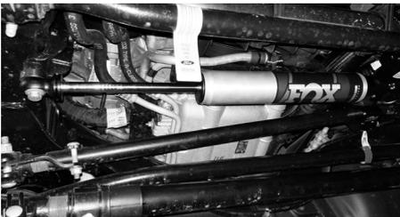
Fig. 3: TS stabilizer clamped to drag link
