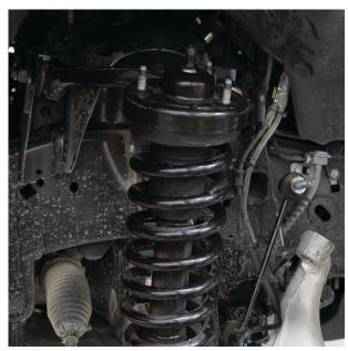
Fig. 6: Free the coil-over.
