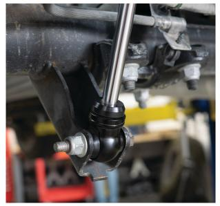
Fig. 16: Install the lower shock bolt.
