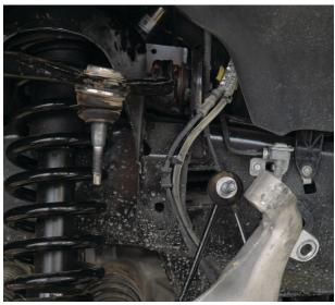
Fig. 4: Separate the UCA and upright.
