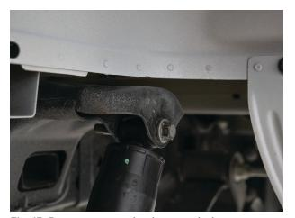
Fig. 13: Remove upper shock mount bolt.
