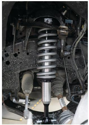
Fig. 8: Install FOX coil-over.
