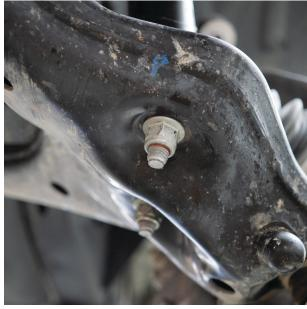
Fig. 7: Remove the bar-pin bolts.
