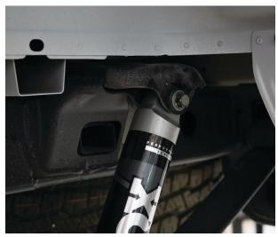
Fig. 15: Install the upper shock mount.
