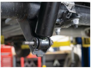
Fig. 14: Remove lower shock mount bolt.
