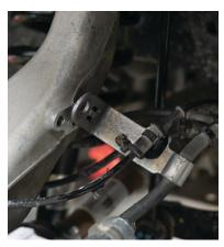
Fig. 1: Brake line bracket.
