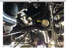
Re-install the track bar and sway bar ends.
