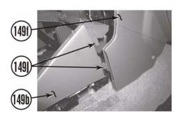
b. Install storage console (149b) on cab (125) with six screws (149i).
