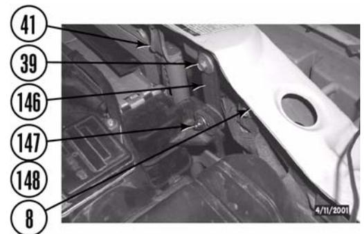
n. Install fan shroud (40) on radiator (41) with two bolts with captive washers (39). Do not tighten.
