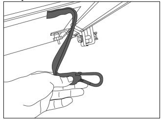
When installing the side rail, make sure one side rail clamp (1-H) is installed nearby the Strap Safety Buckle position. There is a hole on the bottom of the clamp. Snap the safety buckle into the hole of the clamp.
