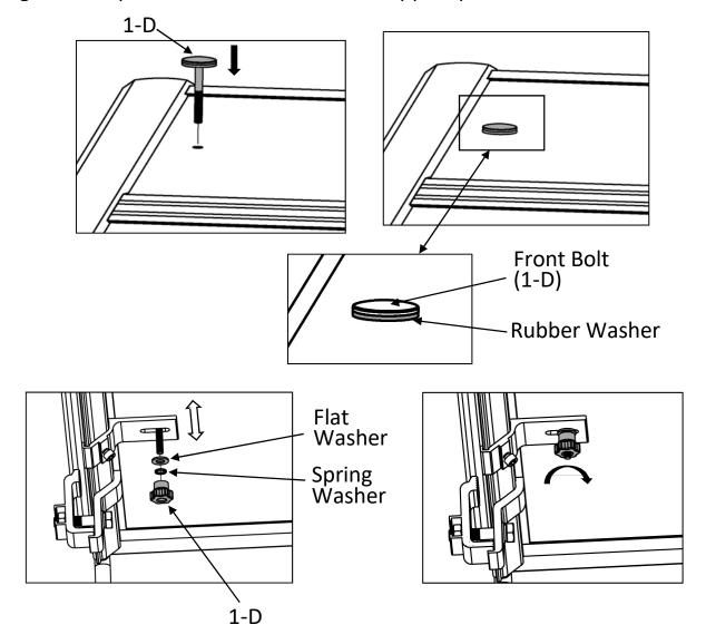
**ATTENTION**: Make sure the Flat Washer and Spring Washer are all placed on bolt before screw the plastic nut on.
