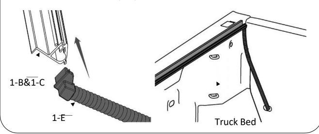
Cut the Rubber strip into six (or more) pieces. Some truck bed edges are not flat, so you need to stick the rubber strips on the side rail's upper or lower edges.
