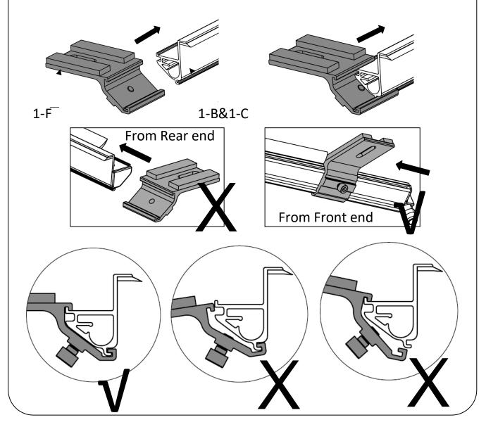
2-2 Slide the Side Rail Locking Latch (1-G) into side rail (from rear end) and move it to the rear part of side rail. Do not tighten the bolts.
