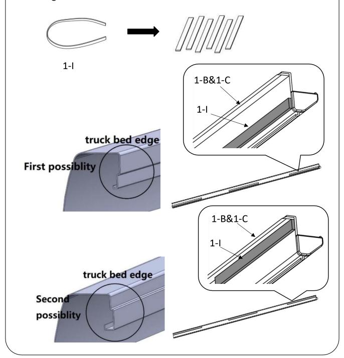
Place the side rail on the bed rail, and push it to the front wall of truck bed. Place one clamp (1-H) at the front of the side rail and one at the rear (please make sure the rear clamps is placed on the position that is closest to tailgate). Tighten the clamps each side. \*For 6.5' beds, an additional clamp will be used at the middle of side rail.
