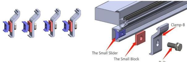
Step-1. Insert the small sliders into the Track Channels. Place one in the front of channel and the other one in the rear of the channel. \*For 6.5' bed, an additional slider will install in the middle of channel.
