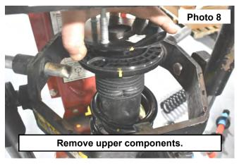
14. Once the spring seat is loosened, remove the end cap, rubber spring isolator and spring seat. Retain for reuse. **See Photo 10.**
