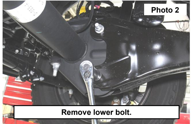
5. Remove the lower radius arm bolt using a 24mm wrench and socket. **See Photo 2.**
