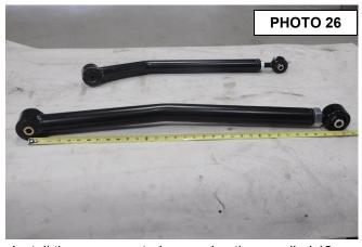
34. Install the upper control arm using the supplied 12mm x 180mm bolt, washers, and lock nut (78630BAG2). Do not tighten at this time. **See Photo 27.**
