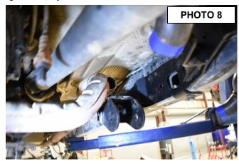
14. Place the cutout portion of the exhaust back into place. You will need to slightly rotate this section so that it is not coming into contact with the new control arm bracket. **2010-2011 Models—** Make sure the O2 sensor is not making contact with any part of the Jeep. **See Photos 9 & 10.**
