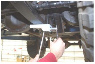
17. Install new brake lines in stock hole locations reusing the T45 torx head bolt on frame rail for the new supplied bracket.
