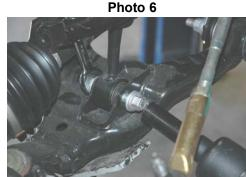
9. Install the new strut extension bracket. Align the holes on the strut extension with the bolts on top of the strut plate and secure with factory hardware. Torque fasteners. **See Photo 7**.
