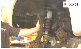
**Install Lifted Knuckle Using Stock Hardware**
