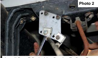
Install Rear E Brake Line Bracket To Rear Frame
