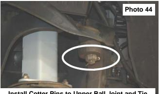
Install Cotter Pins to Upper Ball Joint and Tie Rod Ends
