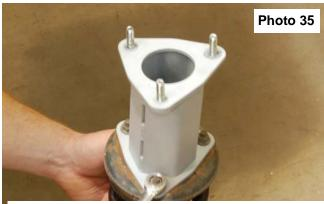
Install Strut Spacer on Strut with Shorter Side to Back
