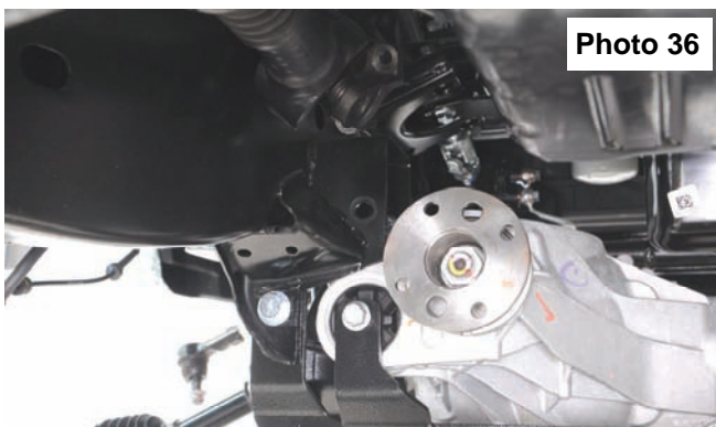
Bolt rear crossmember to differential.
