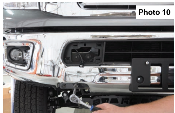
Remove the front bumper mounting bolts.
