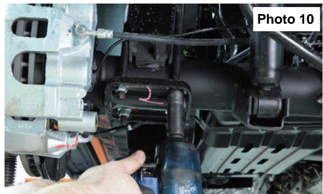
Remove the factory u bolts and hardware.
