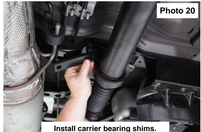
Install carrier bearing shims.
