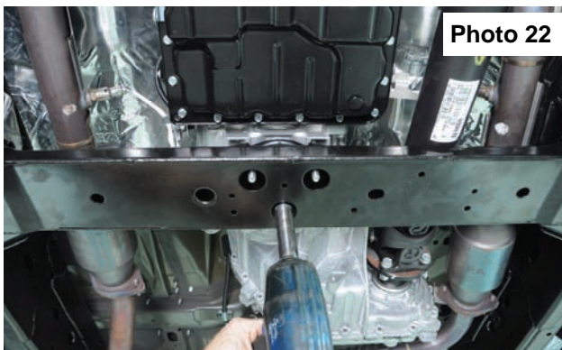
Remove transmission mount nuts.
