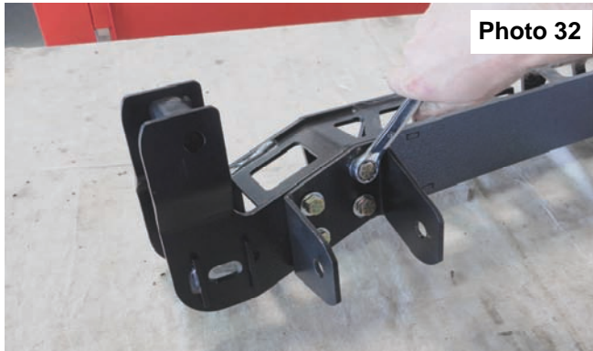
Install differential drop brackets on front crossmember.
