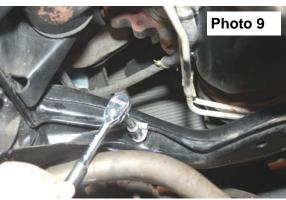
stall the new track rod bracket in stock mount with flat washer in between the bracket and the stock mount as shown with supplied 18mm x 70mm bolt, washer/nut. Tighten using a 1 1/16 wrench. **See Photo 10.**
