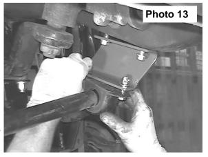
If the vehicle you are working on is equipped with a stock steering stabilizer, remove the stabilizer from the stock location. Because of the pitman arm location you will not be able to reuse the stock steering stabilizer. Rough Country offers a replacement and a dual stabilizer part #87321 that can be used for this application. Call your local Rough Country dealer for more information.
