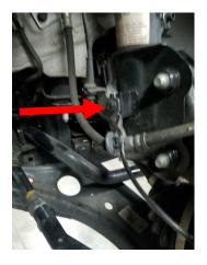
With an adjustable jack under the lower control arm, remove the strut to knuckle fasteners. Retain factory hardware.
