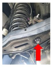
Loosen but do not remove the rear alignment cam bolts.
