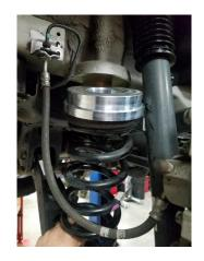
Position the spring spacer with the nipple on the vehicle body. The spring seated on the lower control arm spring isolator.
