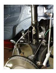
Remove the upper strut hardware. Make sure to hold the strut assembly from falling out of the vehicle. A helper is recommended for removal.
