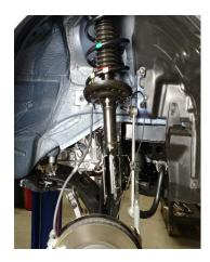
Raise the knuckle up and install into the strut body. Install the bolt into the upper hole and the remaining bolt into the lower. Torque to 90ft-lbs.
