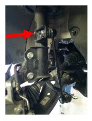
Remove the brake line bracket and ABS wire at the strut body. Let hang out of the way. Retain factory hardware.
