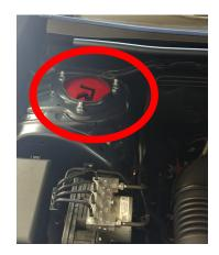
Install the completed strut assembly to the strut tower using the provided M10 flange nuts. Leave loose to aid in installation of the knuckle. A helper is recommended.
