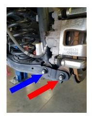
Reattach the rear brake line bracket to the frame using the factory hardware torque 10ft-lbs.
