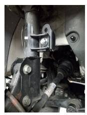
Add the End Link ball joint spacer to the sway bar end link. Attach the sway bar end link to the previous installed bracket with the spacer between the end link and bracket. Use factory hardware torque to 65ft-lbs.
