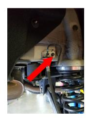
Remove the fastener that connect the rear sway bar end links to the lower control arm.
