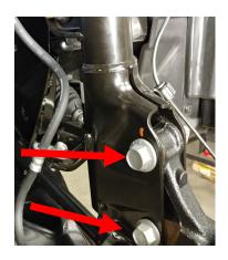
Reattach the ABS and brake line bracket to the strut body. Torque to 5ft-lbs.
