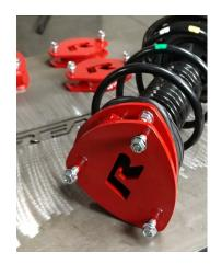
When installed correctly, the R logo will be legible through the strut tower when facing the engine compartment from the side that you are on. Passenger side shown. The spacers are offset to the inside and rear of the vehicle to adjust for camber and caster. THEY MUST BE INSTALLED AS SHOWN.
