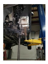
Remove the factory sway bar end link from the strut assembly. Retain factory hardware.
