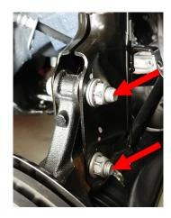
While keeping the lower control arm supported, release the knuckle from the strut body and let hang out of the way. Make sure to not overextend the ABS, brake line, and CV axle. Adjust as necessary.
