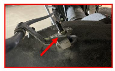
Install the provided e-brake bracket extension to the factory bracket with the provided hardware.
