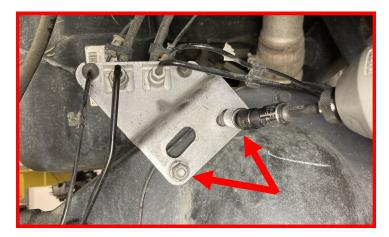
Remove the brake line twist retainer on the backside of the differential cover.
