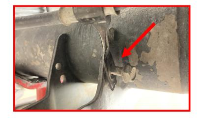
Remove both frame and axle shock mounting bolts. Remove shock from vehicle.
