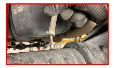
Install the rear shocks upper and lower mounting locations on both driver and passenger side using the factory hardware.
