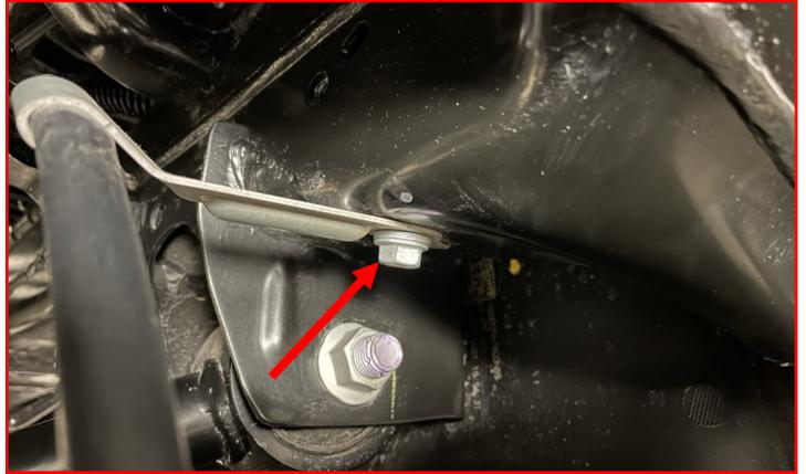
Remove the **bolt** holding the brake line to the frame.
