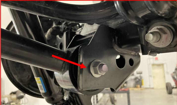
Loosen but **DO NOT** remove the **lower shock bolt**.
