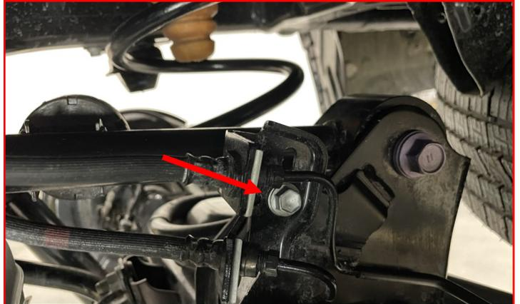
Remove the **end link nut** and let the end hang out of the way.
