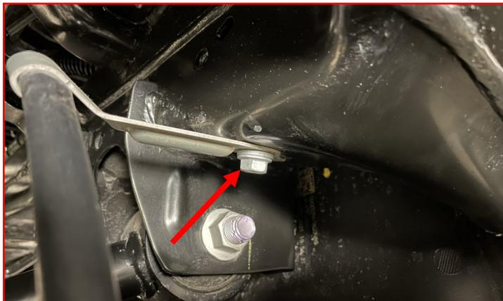
Install the **bolt** holding the brake line to the frame.
