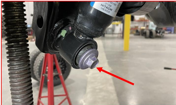
Remove the **upper shock nut** and bushing.
