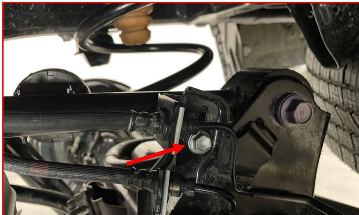
Install the **bolt** (one on each side) holding the brake line to the body using the factory hardware.
