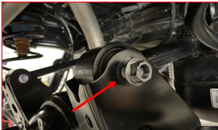
Install the **shock**, **upper factory shock bushing** and **nut**.
