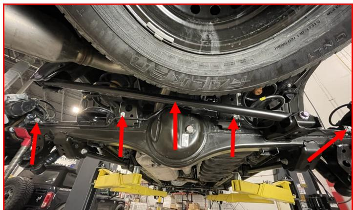
Install the **bolt** (one on each side) holding the brake line to the axle using the factory hardware.
