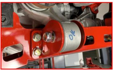
Tighten passenger differential drop bracket hardware.
