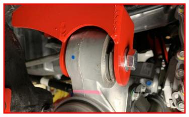
Tighten driver differential drop bracket hardware.
