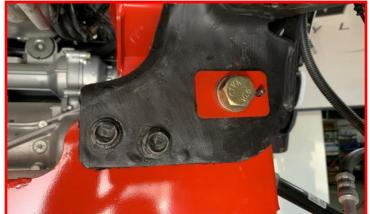
Using the factory cam bolts, cams and nuts, install the lower control arms in the factory orientation. Do not tighten at this time.
