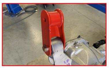
Install differential drop bracket crush sleeve in the factory differential frame mount located on the passenger side. Make sure the crush sleeve is fully inserted prior to installing the differential.
