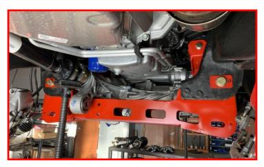
Install the (2) factory rear crossmember bolts and nuts and supplied cam block off plates, M18 bolt, washers and nut through the passenger side factory mount and replacement crossmember. Do not tighten hardware as this time.
