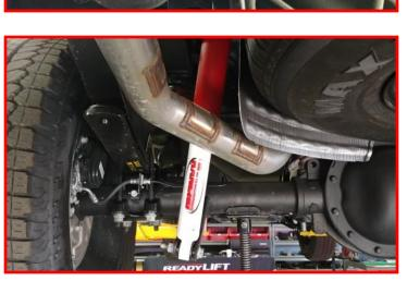
Remove the driver side U-bolts completely and discard. Lower the axle enough to ensure clearance to install lift block making sure that all brake lines and ABS lines do not get over extended.
