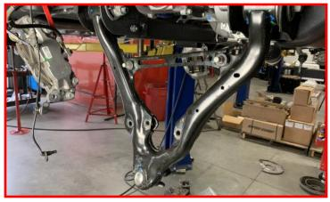
Mark the driveshaft to pinion flange location. Remove the front driveshaft hardware from the flange. Let driveline hang out of the way. Retain the factory hardware.
