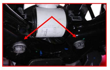
Remove the (3) top strut mounting nuts located on top of the strut tower. Remove strut assembly from vehicle. Retain the factory hardware.
