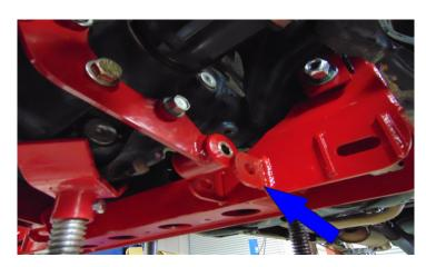
Lower the axle and differential down to the passenger side bracket start the original factory bolts, do not tighten. Rotate the driver side bracket to the differential add the three laser cut washers between the bracket and the differential use the original factory bolts to fasten. Do not tighten at this time.
