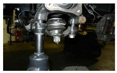
Remove lower strut hardware. Loosen the lower control arm (LCA) cams and let the LCA swing out of the way.
