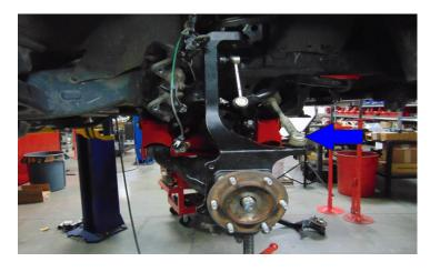
Tighten and torque the front and rear crossmember.
