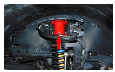
Raise the lower control arm and fasten to the lower strut, use factory hardware hand tight only.
