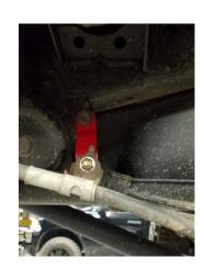
Parking brake clarification: The straight/flat bracket attaches near the spring perch toward the front of the spring. The Z shaped bracket mounts closer to the tire/mid spring.
