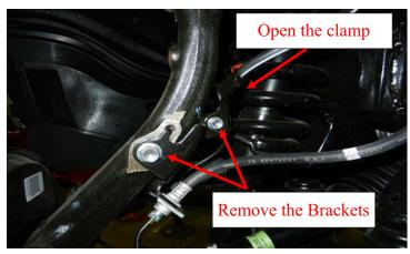
Remove the wheel speed sensor from the steering knuckle.
