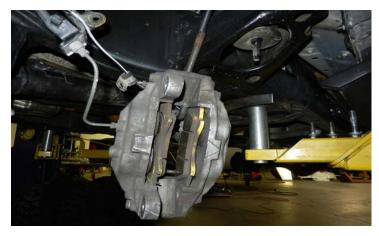
Remove the safety clip from the upper ball joint, cotter pin from the tie rod ends, and axle nut.
