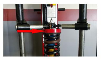
Add the strut spacer to the strut assembly making sure the alignment notches on the spacer face to the out side of the wheel well when installed on the vehicle. Use factory hardware torque 35 ft-lbs
