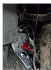
Attach the OEM ABS wire bracket to the ReadyLIFT steering bracket use factory hardware torque 10ft-lbs. Install the wheel speed sensor to the ReadyLIFT steering knuckle. Use the factory hardware torque 5 ft-lbs. Adjust the ABS wire as necessary, attach the ABS wire to the bracket use the factory clip.
