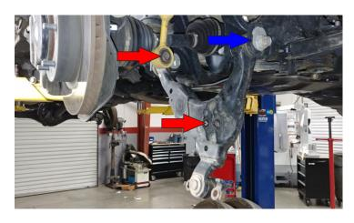
Remove the LCA from the vehicle. Loosen but do not remove the upper control arm. Hold onto the strut, remove the upper strut hardware, remove the strut from the vehicle.
