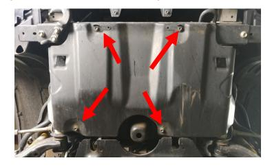
Remove the differential gravel guard.
