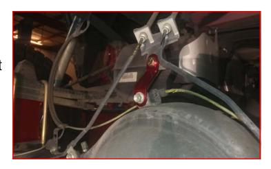
Flip the 2 factory clamps to the left and right of the center mount over and install using factory hardware. You may have to gently pull the metal brake lines through the outer clamps to gain adequate clearance. Torque to 5 ft-lbs.
