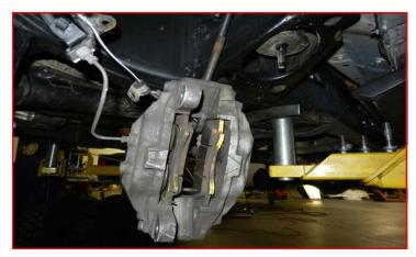
Remove the safety clip from the upper ball joint, and cotter pins from the tie rod ends, and axle nuts.
