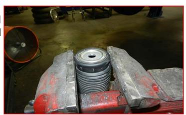
Use a suitable cutting tool and remove the tip of the shock to the first thread. Sand the cut to remove any burs.
