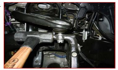
Remove the lower ball joint cradle from the knuckle. Remove the knuckle from the vehicle.
