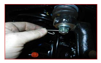
Remove the axle nut safety keeper and then remove the axle nut.
