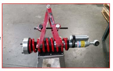
Install the ReadyLIFT strut extensions to their corresponding sides using factory hardware. D and P are cut into the top plate. D is for driver and P for passenger. Continue installation as normal for the rest of the front.
