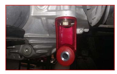
Install the ReadyLIFT rear cross member using M18 x 150mm bolts, washers, cam block off plates, and clock nuts. Do not tighten at this time.
