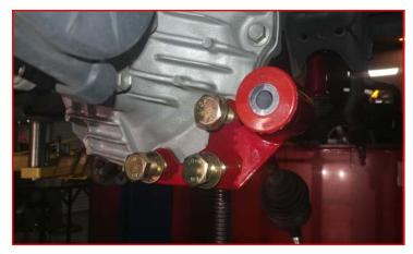
Install the ReadyLIFT drivers side rear mount onto the differential using M14 x 25mm bolt, and washer. Do not tighten at this time.
