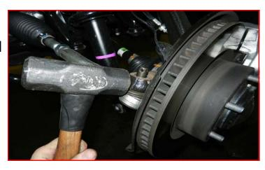
Mark a line 1/4" from the end of the inner tie rod and using a suitable cutting tool, remove outer marked section. Clean any burs from the cutting process. Install the outer tie rod end from the opposite side.
