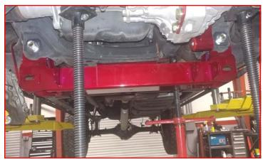
Install the ReadyLIFT front cross member using 7/8" x 5.5" bolts, washers, cam block off plates, and clock nuts. Do not tighten at this time.
