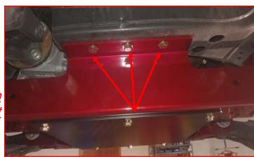
Install the ReadyLIFT skid plate to the cross members using 3/8" x 1" bolts, and washers. Torque to 30 ft-lbs.
