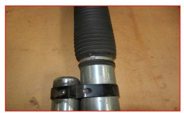
Remove the boot from the shock and place in a vice or suitable clamp. Drill out the top of the boot washer to 11/16".
