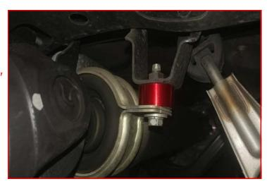
Tighten the upper shock hardware but do not over tighten as you are just setting about 1/4 crush on the rubber bushings (see picture for proper crush). Torque the lower shock hardware to 45 ft-lbs, and ubolts to 110 ft-lbs. Have a reputable alignment shop set the alignment to the provided alignment specs on the last page of the instruction booklet.
