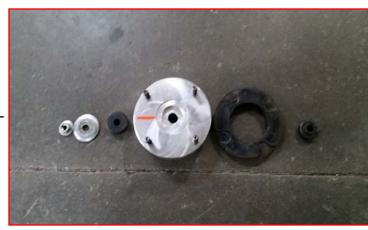
Remove the rubber bushing from the factory top hat. The inside bushing is glued in place and requires separation. Install in the same order as removed from the factory parts. Install the strut hat in the same orientation as the factory (mark on the top of the top hat indicates outward same as factory top hat) using the factory hardware. Torque to 30 ft-lbs.
