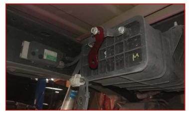
Install the ABS bracket to the Ready-LIFT extension (Z shaped) using 5/16" x 1" bolt, washers, and c-lock nut. Torque all to 5 ft-lbs.
