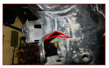
Torque the front cross member bolts to 200 ft-lbs, rear cross member bolts to 150 ft-lbs, 1/2" diff hardware to 95 ft-lbs, and M14 differential hardware to 80 ft-lbs.
