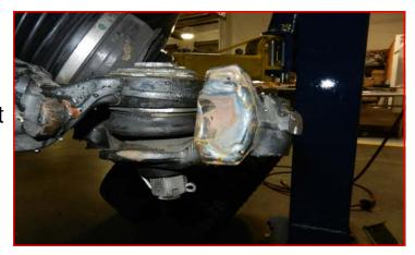
Install the ReadyLIFT knuckle to the upper ball joint and lower ball joint cradle (while positioning the axle through the dust seal and hub bearing) using the factory hardware. Add a drop of thread locker to the lower mounting hardware.
