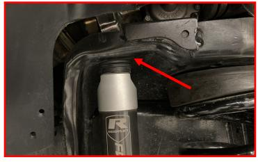
Install the Falcon front shock lower mount to the axle mount.
