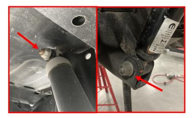
Install the rear Falcon shock upper mount onto the frame using the factory hardware.
