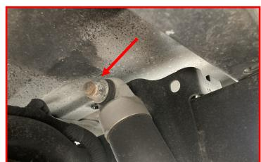
Install the rear Falcon shock into the axle mount using the factory hardware.
