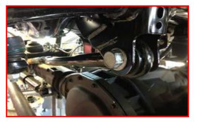
Loosen the rear radius arm bolt.
