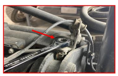
Loosen track bar bolts at the frame and axle ends.
