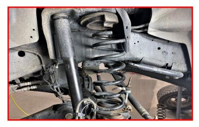
Remove the factory spring isolator.
