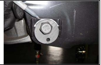
3 ) Remove the 24mm lower control arm nuts and bolts.
