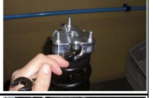
5 ) Install strut back into the factory position. (The strut will install 180 degrees from the position that it was removed.)
