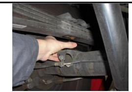
Install the ReadyLift® 1" rear block. Lower the jack and make sure that the leaf spring center pin goes into the hole on top of the block.
