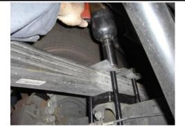
Install ReadyLift® u-bolts using the hardware provided. Torque to 120 ft/lbs. Repeat on opposite side.
