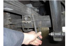
Remove the two u-bolts. Using a jack and a block of wood, carefully raise the truck by the leaf spring until the OEM block is loose and there is enough room for the new block.
