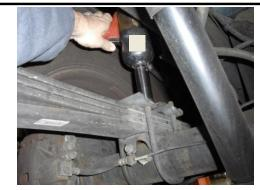
**REAR BLOCK INSTALLATION** Remove the four 21mm nuts.
