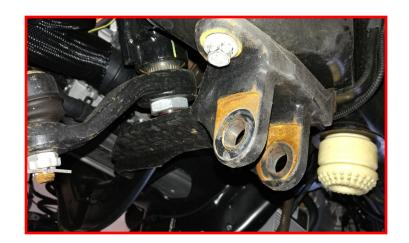
Install the ReadyLIFT track bar bracket to the frame using factory hardware. Torque to 95 ft-lbs. Install the track bar to the ReadyLIFT bracket using factory hardware. Lower the vehicle to the ground for torque. Torque the track bar hardware to 250 ft-lbs.
