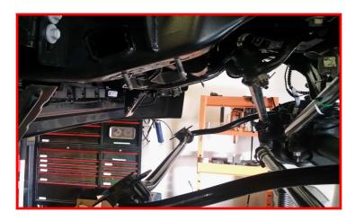
Loosen but do not remove the radius arm bolt at the frame. Lower the axle enough to remove the front springs. Make sure not to over extend the ABS, brake lines, and vent tube. Install the ReadyLIFT urethane isolator, spring spacer, and then factory rubber isolator onto the spring. Raise the axle enough to hold the spring assembly in place.
