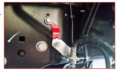
2011 - 2016: The ReadyLIFT extension lower bolt holes are offset. The offset hole will be closest to the radius arm. Install the shock extensions to the axle using factory hardware and the shock to the shock extensions using the M12 x 70mm bolt, washers and nuts. Do not tighten at this time.
