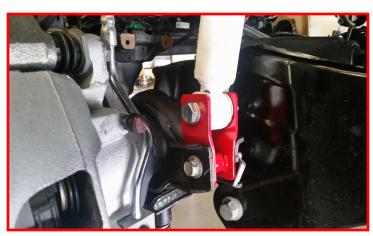
Remove the factory bump stop by pulling it out of its mount. Remove the mount from the frame by pulling it out of its mount.
