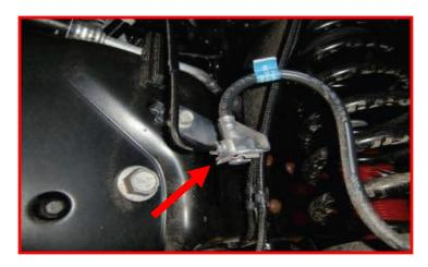
2017 - UP front brake line: Remove the brake line bracket at the frame. Remove the brake line bracket at the axle.
