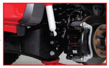
Install the ReadyLIFT shock extensions to the axle using factory hardware making sure the offset hole is towards the rear of the axle. Install the shock to the Ready-LIFT shock extensions using the M14 x 70mm bolt, washers and nuts. Torque to 45 ft-lbs. (2017 and up models shown, earlier models differ slightly. The offset hole will end up towards the radius arm.)
