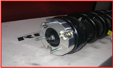
Install the completed strut into the side of the vehicle they came out of using provided 10mm flange nuts. Do not tighten at this time.
