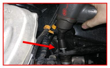
Remove the CV axle nut cover.
