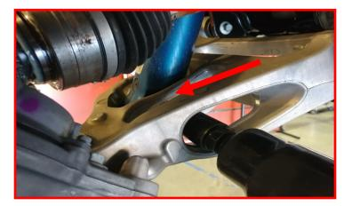
Remove the upper strut mount at the frame and remove the strut from the vehicle. Mark the top hat and lower spring perch in relation to the strut body. This is very important to keep the spring to upper control arm clearances for full droop.
