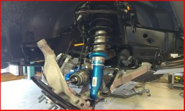
2019 and UP Models: be careful not to damage the electric motor and harness when removing from the vehicle.
