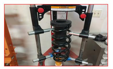
2.5" kit Pre-load spacer: Install the Ready-LIFT spring spacer into the top hat.
