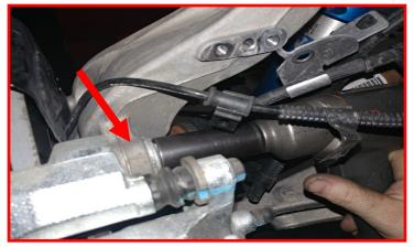
Use a suitable hanger, hang the caliper out of the way. Never let the caliper hang from the rubber line. Remove the rotor from the hub.
