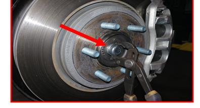
Remove the CV axle nut.
