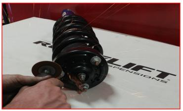
**1.5"** and **2.5"** kit top extension: Install the ReadyLIFT strut extension using provided 10mm flange nuts. Torque to 15 ft-lbs.
