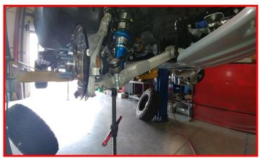
Lower the upper control arm while lining the upper ball joint into place. Install the upper ball joint to the knuckle using factory hardware. Torque to 65 ft-lbs.
