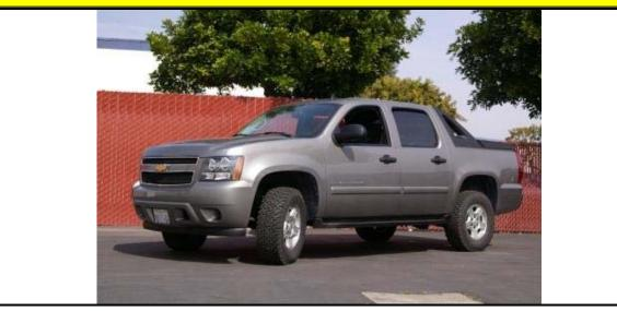
After ReadyLift® 66-3085 and 66-3010. 285/70R17 tires mounted on Factory wheels.
