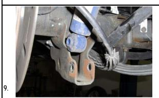
Remove the 21mm lower shock mount bolt on both sides.
