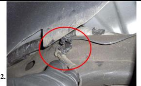
Unhook the ABS line at the frame on the both sides.
