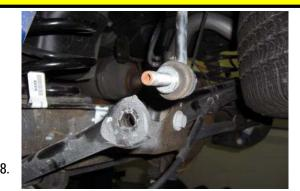
Use a jack to support the axle, this will allow you to lower and raise the axle as you need during installation. Unbolt the lower sway bar end link on both sides with a 17mm wrench.
