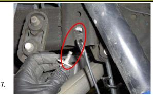
Remove the 13mm emergency brake line support bracket on the passenger side frame rail.
