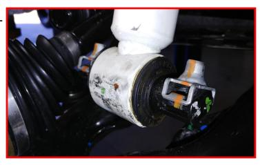
Remove factory upper control arm from vehicle and **discard factory arm.**
