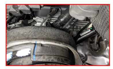
Torque strut to lower control arm bolts to 45 ft-lbs.
