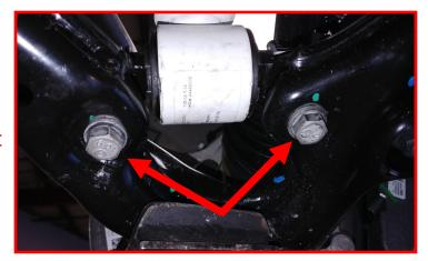
Remove lower sway bar end link nut.
