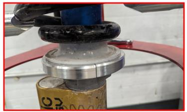
Relieve the spring pressure and remove from spring compressor.
