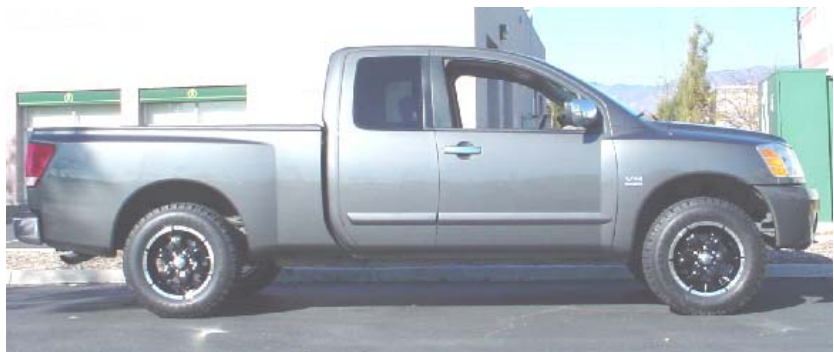
Nissan Titan with ReadyLift ® and 295 / 70x17 tires installed on 17x8.5 wheels with 4.5" backspacing
