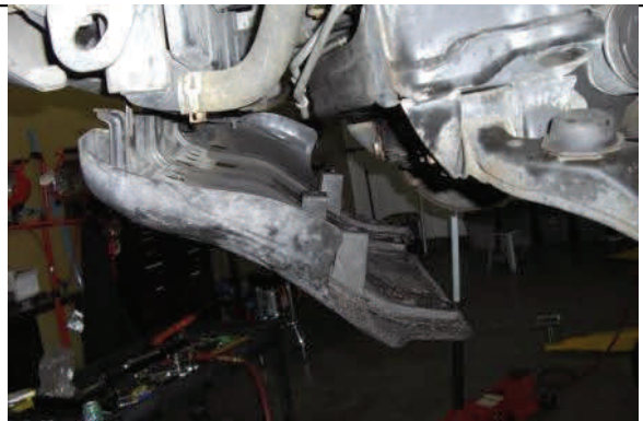
4WD models and 2.5-3.0" kits remove front skid plate
