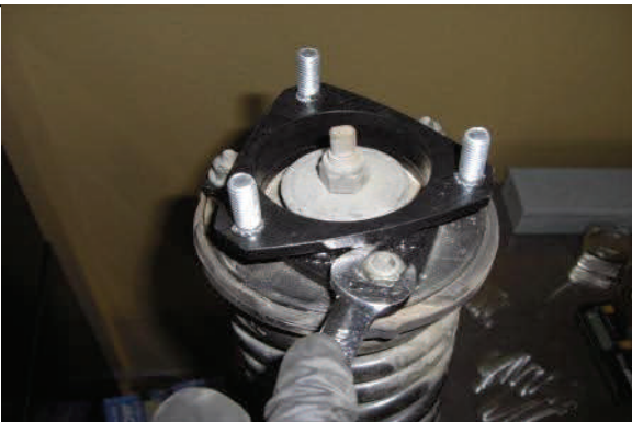
Attach new strut extension with OE hardware
