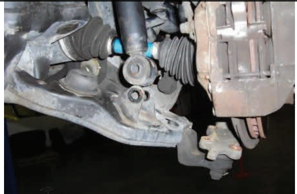
Lower control arm if necessary to install lower mount
