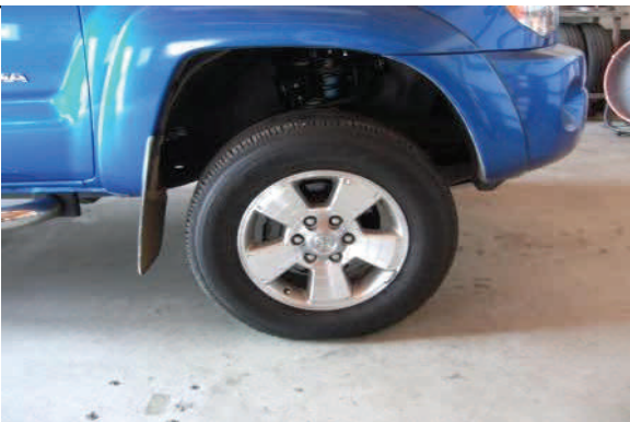
Reconnect sway bar links, install wheels/tires torque to spec.
