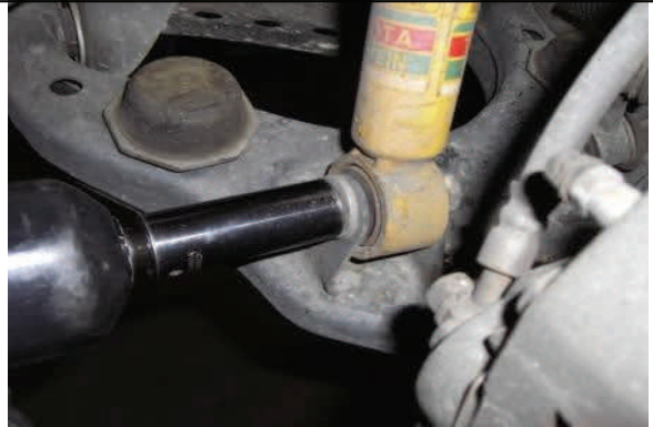
Disconnect lower strut mounting hardware
