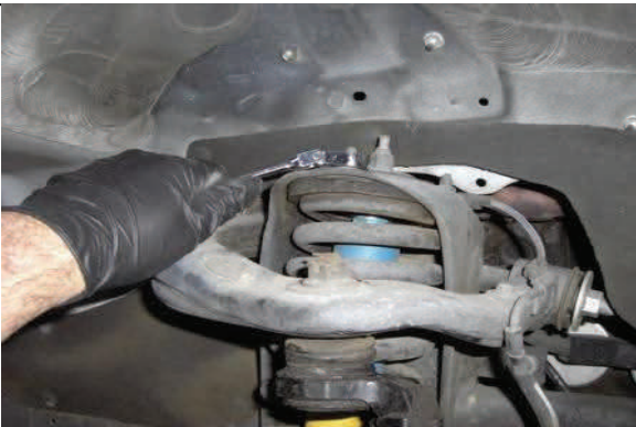
Disconnect upper strut mounting hardware
