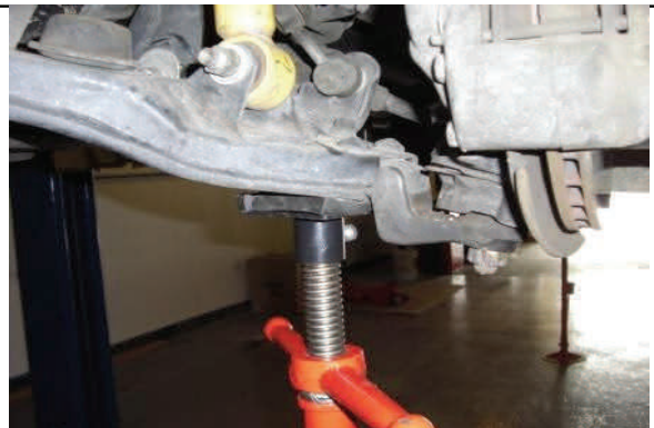
Raise lower control arm and attach lower strut mount
