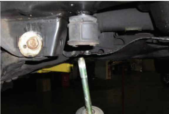
4WD Support differential and remove (2) front mounting bolts
