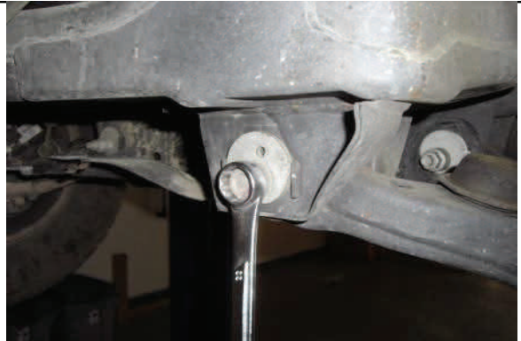
Reset and tighten lower control arm bolts
