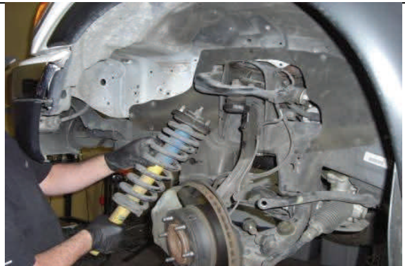
Remove strut from vehicle
