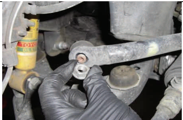
Reconnect sway bar end links. Move to the rear installation
