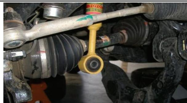
3. Loosen, but do not remove the 19mm lower control arm nut and bolt, Remove the 19mm lower ball joint bolts.
