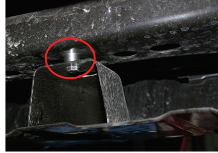
Using the hardware provided, install the M8 bolt, washer, skid plate, and 1/2 tall spacer into the back two skid plate mounting points. Use the OEM hardware for the two front mounting parts.
