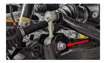
Loosen, but DO NOT REMOVE the upper control arm bolt.
