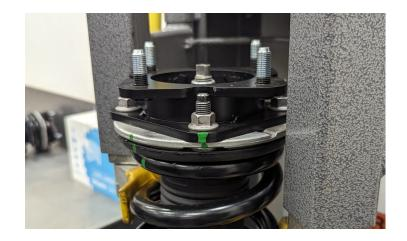
Compress the spring and rotate the top hat and ReadyLIFT front strut spacer so that the mark made in the previous step aligns with the mark on the spring.
