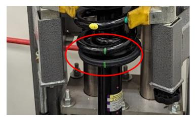
Install the strut assembly back into vehicle using the provided M10 flange nuts.
