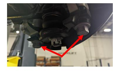
Remove lower control arm to strut bolt.
