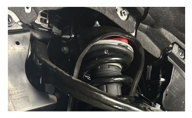
Install the lower strut bolt and nut.
