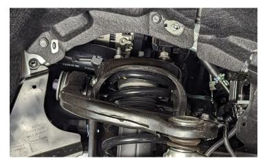
On the strut top mount, measure and mark 3/8" from the top of each stud.
