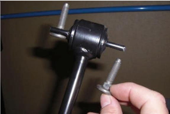
Remove both bolts and use new provided hardware
