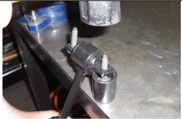
Hammer out OE mounting bolts
