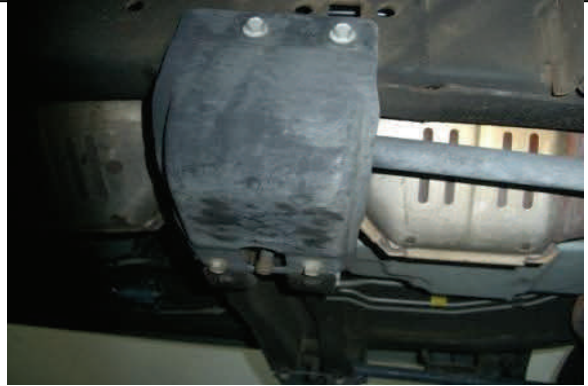
Locate cross member cover and remove bolts
