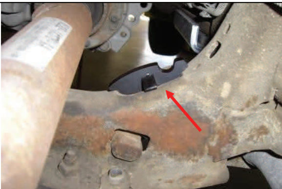
Place torsion bar unloading tool adapter above cross member
