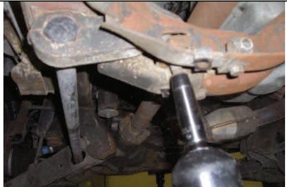
Remove torsion key adjuster bolt
