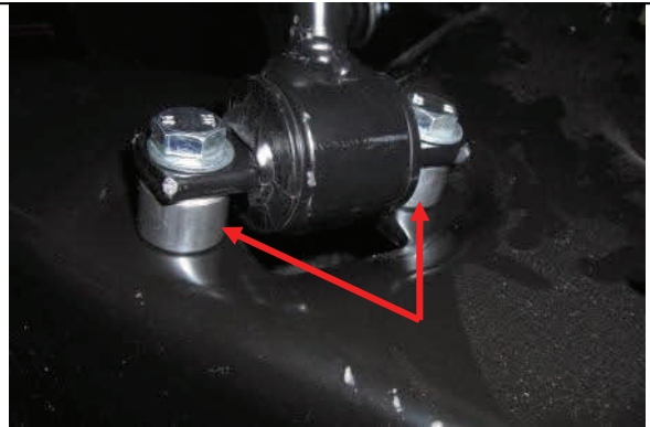
Install shock spacers as shown
