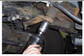
Using a 1 5/16" socket, remove the factory sector shaft nut and lock washer.
