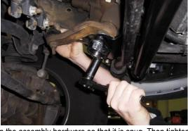
Tighten the assembly hardware so that it is snug. Then tighten the sway bar mounting bolts to 40 lb-ft. Make sure the inner bearing surface can rotate around the sector shaft.
