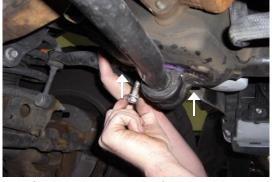
Remove the four bolts that connect the front sway bar to the frame with a 15mm socket or wrench. Hold onto the sway bar while doing this as it will drop when unbolted.
