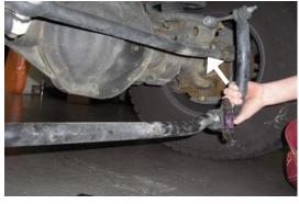
Allow the sway bar to hang down and rest against the crossover bar.
