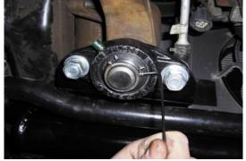
Tighten the bearing assemble hardware to 86 lb-ft. Apply a light thread locker to the set screws and tighten. Make sure the zerk fitting is tight and apply grease using a grease gun.
