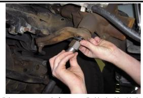
Install the new sector shaft nut supplied in the kit with the factory lock washer.
