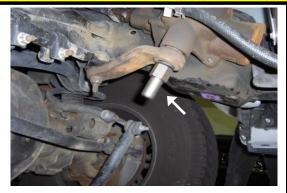
Tighten the new sector shaft nut using a 1 1/4 deep socket. Tighten to 180 lb-ft.
