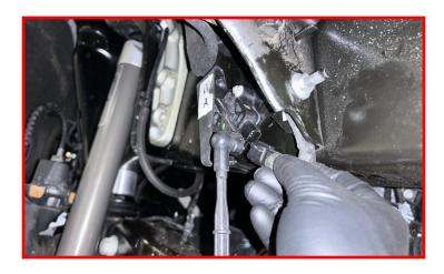
Remove retaining clip from bracket.
