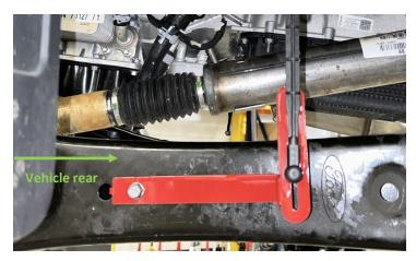
Install headlight leveling link into radius arm bracket.
