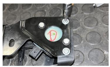
Remove headlight leveling sensor from factory bracket.
