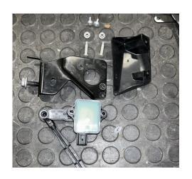
Install sensor onto ReadyLIFT headlight leveling frame bracket with the connection point facing up.
