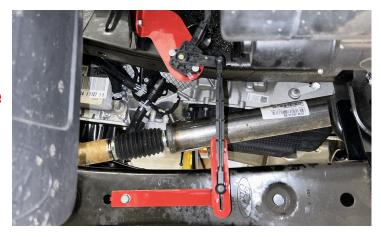
Plug the connector into the headlight leveling sensor.
