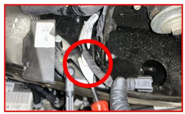
Unclip the sensor wire from the top of the body mount and pull it behind the body mount.
