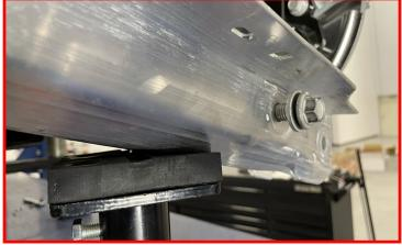
Continue to carefully lift the lower control arm until the factory lower knuckle bolt and lock nut can be installed. Be careful to not lift the vehicle off of the jack stands/ lift.
