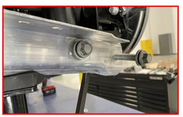
Torque the front trailing arm hardware to 80 ft-lb.
