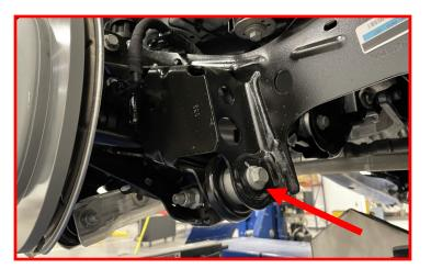
Remove the 15mm Strut and knuckle bolts from the lower control arm. Let the control arm and brake assembly hang.
