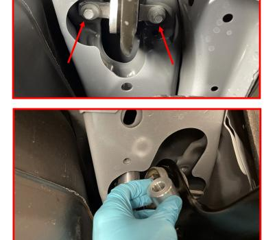
Bolt in the trailing arm using the supplied M14-2.0x60mm bolts, M14 flat washer, and lock washer.
