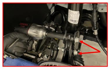
Install the End Link Drop Bracket using the supplied M12-1.25 x 30mm bolt and M12-1.25 Flange Lock Nut Make sure the bolt is installed inboard to outboard.
