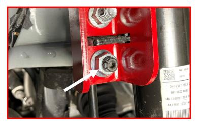
Using factory hardware, reinstall the tie rod.
