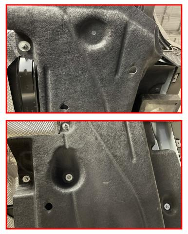
Reinstall the four remaining factory nuts.
