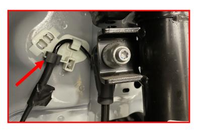
Remove the ABS wire from the strut
