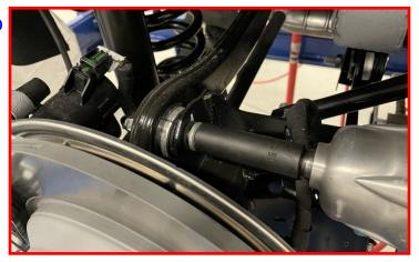
Torque the rear trailing arm hardware to 80 ft-lb.
