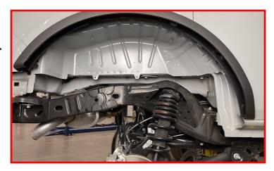
To aid in the removal and installation process, it is best to loosen the rear track bar at the axle.
