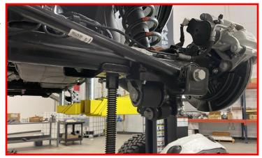
Loosen the (3) top strut nuts.
