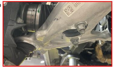
Using an appropriate jack, carefully jack the lower control arm into the frame side pivot pockets.
