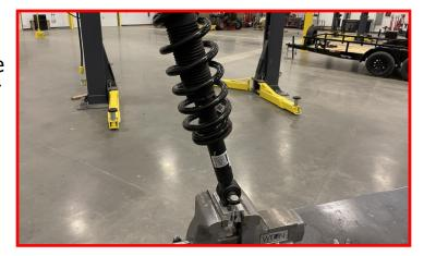
Install the top strut spacer onto the strut assembly using the factory nuts.
