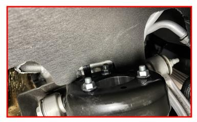
Install the sway bar back into the vehicle in the factory orientation.
