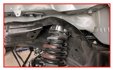
Raise the axle into place and install the lower strut bolts.
