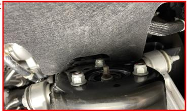
Remove the lower strut nuts.
