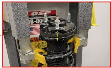
Compress the spring enough to relief pressure on the top hat. Being sure to keep the strut body and upper spring isolator in the factory location, rotate the factory top hat 180 degrees from the previously made marks. This will orient the spring in its original location to prevent the spring from bowing.
