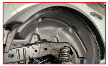
Remove the rear fender liners.
