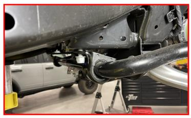
Install the driver and passenger forward sway bar retainer cap bolt.
