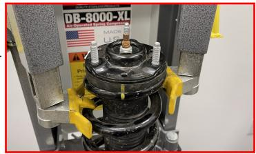
To aid in the installation process clamp the lower strut stud in a set of soft jaws. Using the leverage of the strut, rotate the lower strut bushing 30 degrees in the opposite direction. Effectively orienting the lower strut studs parallel to the strut body.
